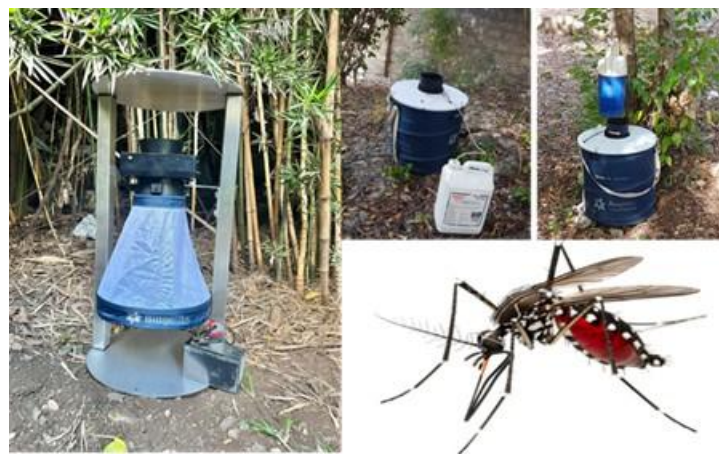
Figure 12: Biogents (BG) Sentinel traps used in NESTLER for survey of adult Aedes mosquito dengue vectors, baited with carbon dioxide as yeast-sugar mixture (left panel) or dry ice (right panel)
