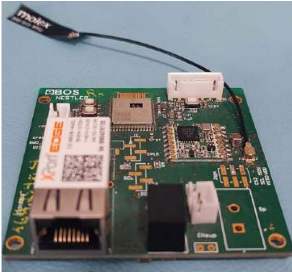
Figure 68: Data Aggregator PCB
