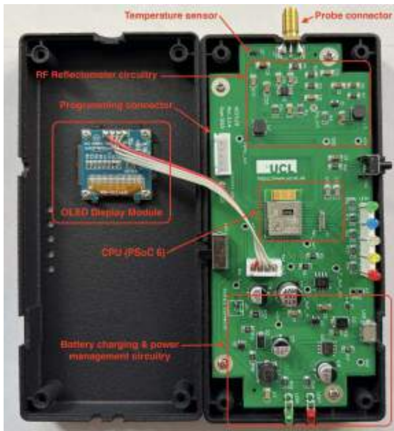
Figure 3: Prototype crop quality measurement device featuring an OLED display and a 5-LED traffic-light indicator system for intuitive visual reporting of crop quality
